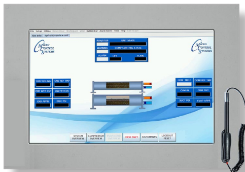
EVAPORATOR CONDENSER OVERVIEW SCREEN
